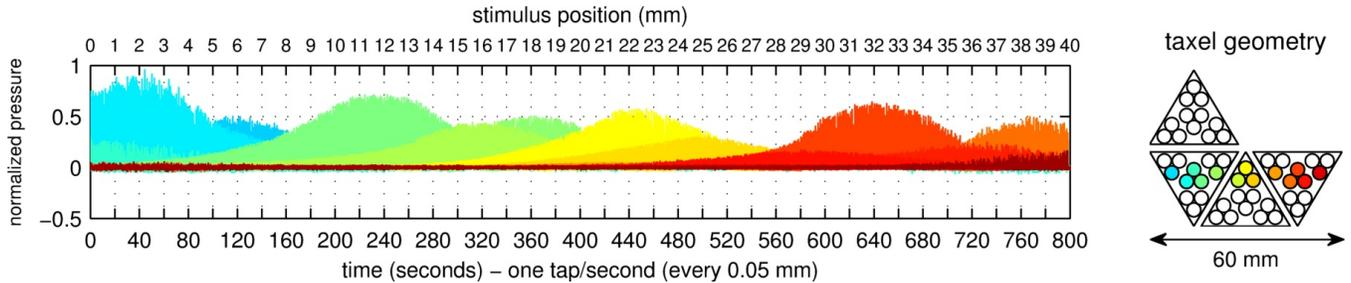
Fig. 4. Tactile data recorded as the tip of a rod (dia. 4 mm) taps against the area of tactile skin at constant rate of 1 tap/second, with 0.05 mm movement after every tap to span a 40 mm range of positions. The color coding of the taxels by their location is shown on the diagram to the right.
