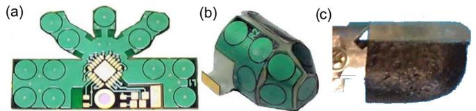
Fig. 1. Construction of tactile sensor shaped like a human fingertip.
