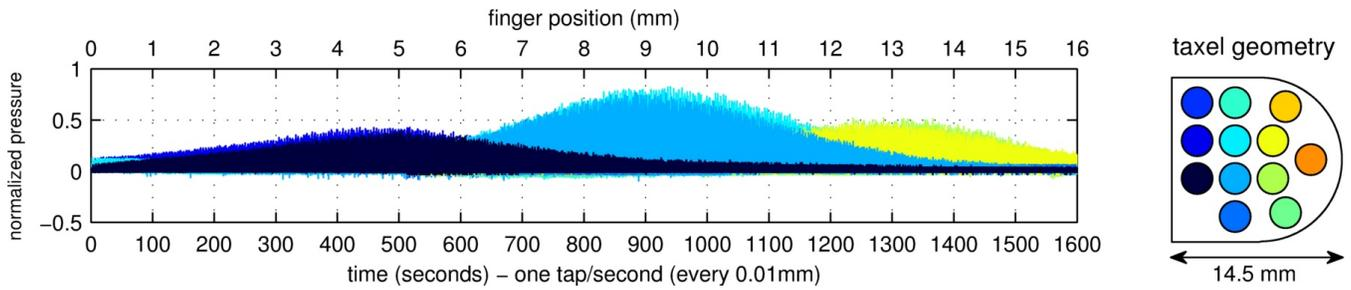
Fig. 3. Tactile data recorded as the fingertip taps against a test rod (dia. 4 mm) at constant rate of 1 tap/second, with 0.01 mm move across the rod after every tap to span a 16 mm range of positions. Taxels are represented in distinct colors depending on the taxel position shown on the diagram to the right.
