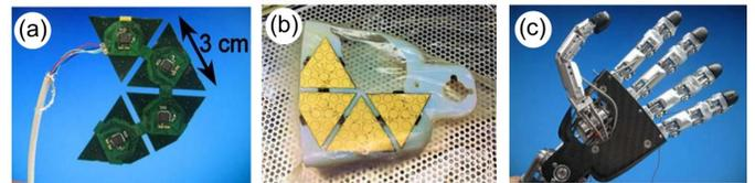
Fig. 2. Construction of area of tactile skin for the palm of a robot hand.
