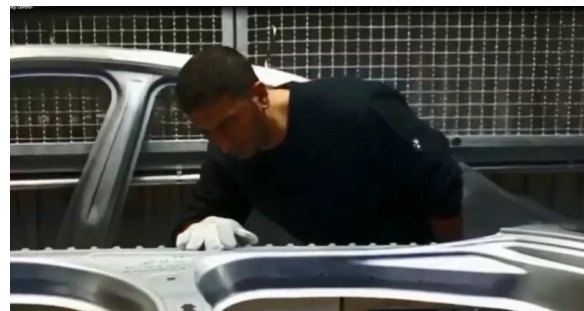
Fig. 2: Tactile quality control on a production line.
