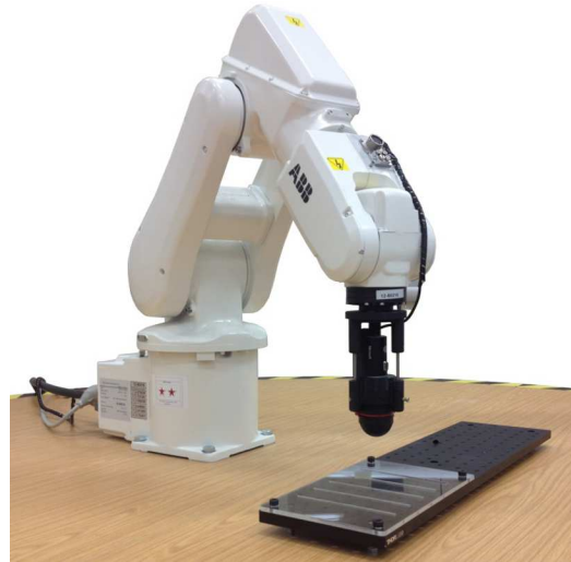
Fig. 1: Tactile quality control robot, comprising a tactile fingertip (the TacTip) mounted as end effector on a robot arm.
